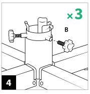
Screw in the large tension knobs into the center collar.
