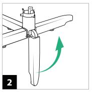
Unfold each of the legs until they have locked into place.
