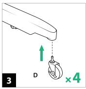
Push the wheels into the leg socket until they lock in place.
