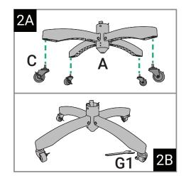
Install wheels. Secure the wheels firmly with the wrench.
