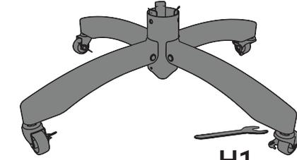
Install wheels. Secure the wheels
