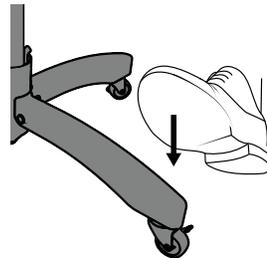
Apply pressure to the stand to keep it stable when pulling up.
